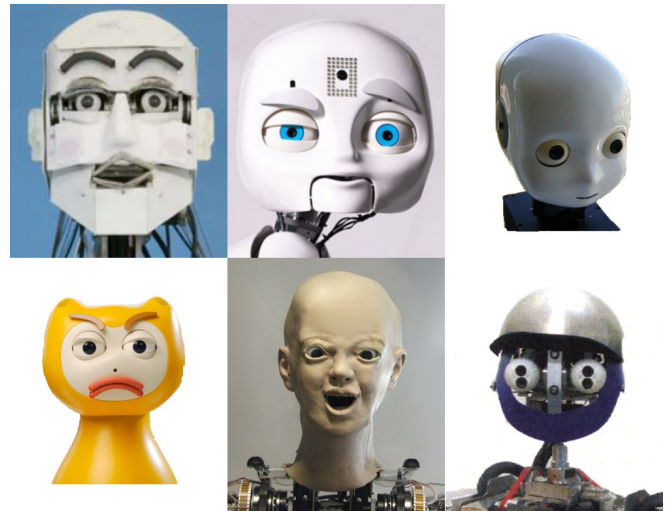
Fig. 2. Heads for comparison. From left to right and top to bottom: WE-4RII, Nexi, iCub, iCat, ANON, Karlsruhe Humanoid Head.
