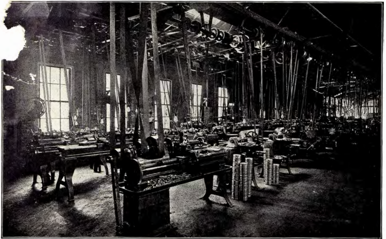
SECTIONAL PHOTOGRAPHIC VIEW SHOWING THE AUTOMATIC MACHINERY USED IN CUTTING THE SPIRAL GEARS AND SPIRAL SHAFTS FOR THE 400 CHAMPION STEEL BLOWERS
