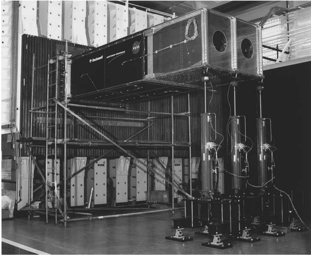
Fig. 11. Composite RLV Wing Box in Test Stand.
