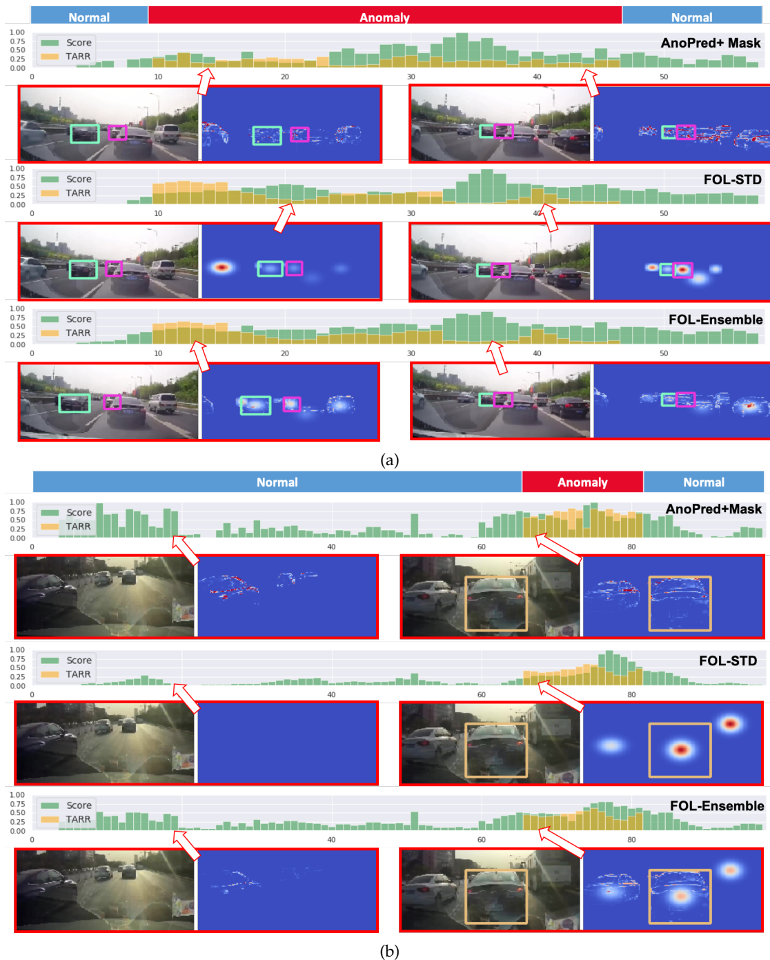
Fig. 9: Per-frame anomaly scores and TARRs of three methods for two different videos. The left and right columns show sample video frames and corresponding score maps, with an arrow indicating their temporal position within the video. Note that TARR only exists in positive frames.
