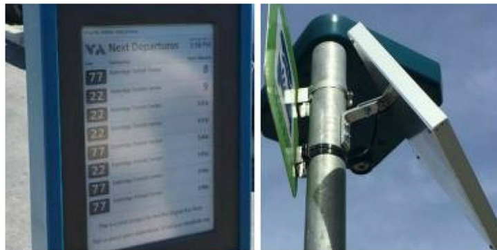
VTA’s new solar-powered real-time information (RTI) signs
