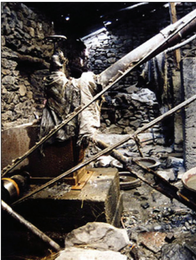
The precarious working conditions, and in particular the use of mercury without any protection nor recovery, are the source of both health and environmental hazards. Photos: MSD
