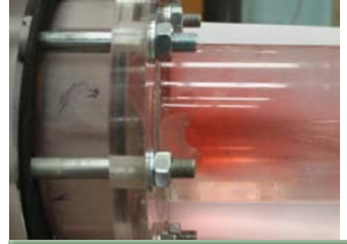
Rapid mixing of additive into the main flow
