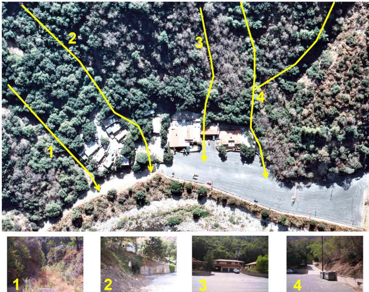
Figure 10: Mapped Drainages that cross the El Encanto Property. Small images show the locations where sediment and water currently traverses the parking lot and road.
