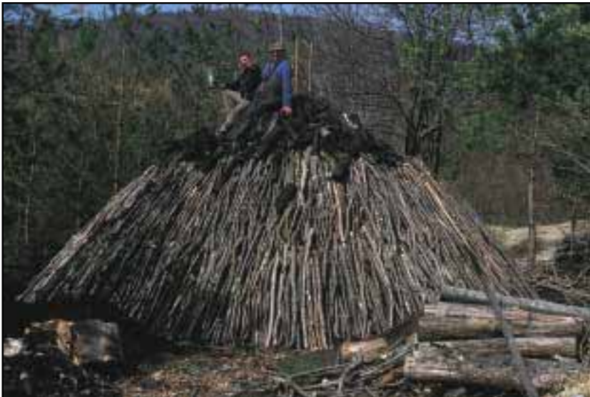
Figure 158. Charcoal burning in the Bena valley. There are still some places in Slovenia where charcoal has been charred in the traditional way.
