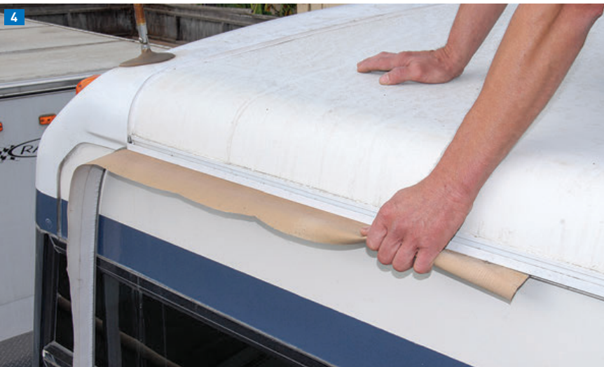
(3 and 4) Loosen the screws that secure the fabric to the roof rail and slide out the remaining awning fragment.
