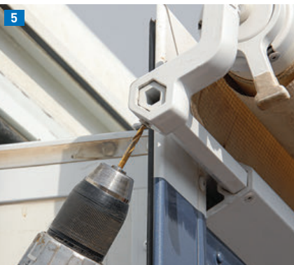
(5) The roller-tube arms are secured to the mounting bracket by a \frac{3}{16} - x \frac{1}{2} -inch aluminum rivet, which must be drilled out. (6) With help from a friend, the tube assembly can now be removed. Even with the rivets drilled out, it might take some wiggling to get the tube free. Hold the tube arm tightly and carefully unwind it, counting the number of revolutions until there is no more tension in the spring. Make sure you mark the direction before unwinding. You'll have to wind on the new material with roughly the same number of revolutions.
