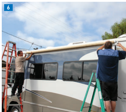
(5) The roller-tube arms are secured to the mounting bracket by a \frac{3}{16} - x \frac{1}{2} -inch aluminum rivet, which must be drilled out. (6) With help from a friend, the tube assembly can now be removed. Even with the rivets drilled out, it might take some wiggling to get the tube free. Hold the tube arm tightly and carefully unwind it, counting the number of revolutions until there is no more tension in the spring. Make sure you mark the direction before unwinding. You'll have to wind on the new material with roughly the same number of revolutions.
