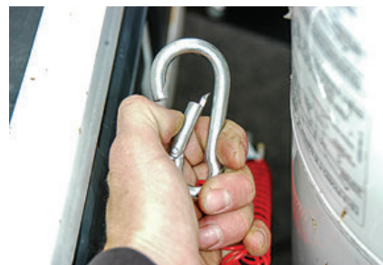
The Coiled Zip breakaway cable hangs neatly when not in use. To connect, the cable is stretched from the switch and attached to the tow vehicle with a carabiner-style spring clip.
