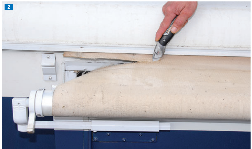
(1) The old slide-topper fabric had been subjected to the elements for years and was practically disintegrating. (2) Rather than slide the old fabric out of the rail, the easiest way is to just cut it with a knife. The slideout was deployed a few inches to create tension in the fabric, after which it was very easy to cut.
