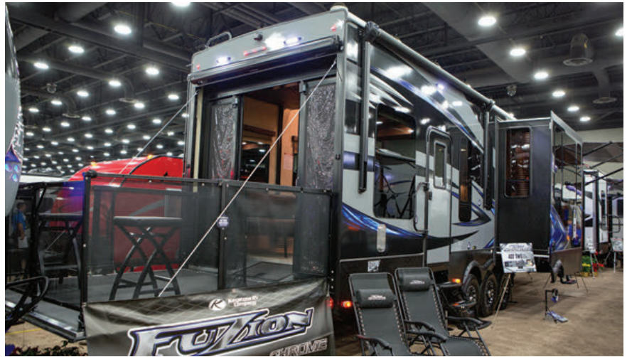
The rear patio was the last great thing to happen to toy-hauler ramp doors, and the Fast-Track patio system, shown on the Keystone Fuzion Chrome, is the newest. Instead of individual rail sections, the Fast-Track assembly stores in the entryway, then simply unfolds and telescopes into place.
