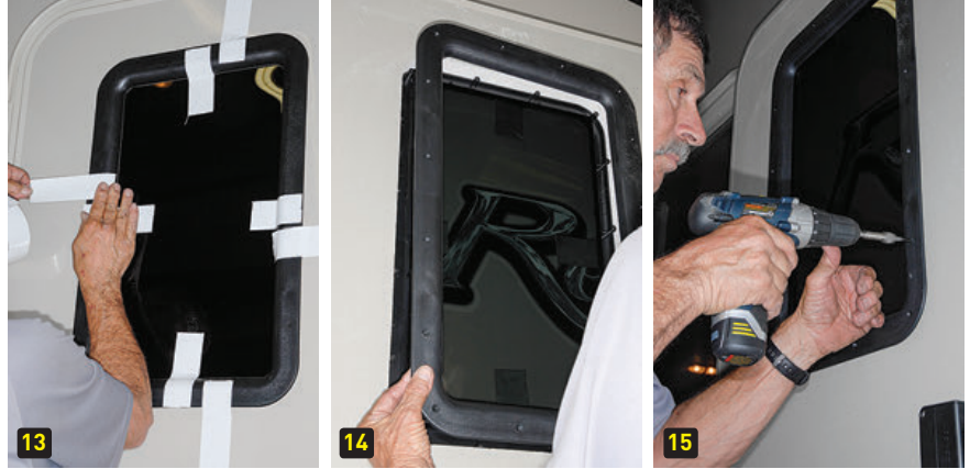
[13] Use duct tape to hold the glass and outer frame in place for a one-person job. [14 and 15] Install the inside frame top side up and do not overtighten the screws. The plastic frame will certainly crack when overtightened.
