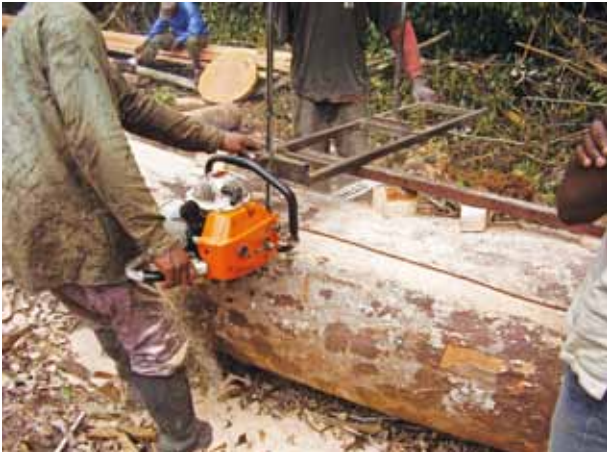
Figure 2. A gruminette for small-scale sawing (Photo by Régis Is-maël Yembe-Yembe)
