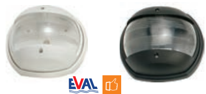
MASTHEAD LIGHT, WHITE Spare glass code PÁ3022. 12V/15W, 225°
