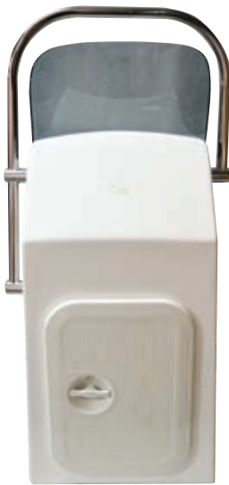
STANDING OVAL CONSOLE With hatch. Made of fiberglass.
