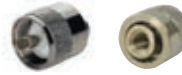
Code 1917-1 MALE CONNECTOR FOR ANTENNA High quality male connector, nickel plated with silver tip and teflon insulator. Suitable for coaxial cable RG 58. Internal diameter 0,6 cm
