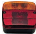
REAR SQUARE LIGHT Three functions: stop - tail - position. Lamps: 2 x 21 W bipolar and 1 x 5 W tube. Available with spare glass code 1534-1.
