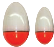
FISHING SENSOR (Bobble) It analyses the vibrations on the fishing line and it lights green when it turns on. It becomes red when it senses a fish bite. Works with a battery CR 1225 with 1000 hour life time that it can be changed. Visible from 90m with auto switch on/off. Water resistant with special mechanism that isolate the waving from 4 grade waves.
