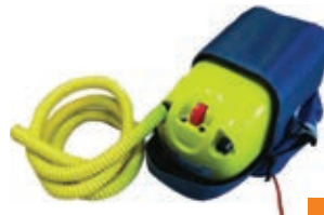
Code 1227 ELECTRIC PUMP 500 lt/min, 12V, Maximum pressure 80 Kpa, Weight 2,6 kg, High speed and high pressure, Equipped with connection clip for batteries and 3 m wire and spiral tube 2 m.
