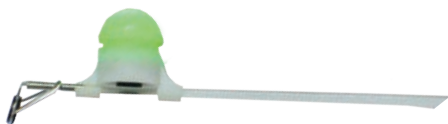
FISHING SENSOR (rod) Easy assembly on the tip of your rod with 3mm and 5mm thickness rods. It analyses the vibrations on the rod and it lights green when it turns on. It becomes red when it senses a fish bite. Works with a battery CR 1225 with 1000 hour life time that it can be changed. Visible from 90m with auto switch on/off. Water resistant with special mechanism that isolate the waving from 4 grade waves.
