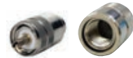
1917-2 MALE CONNECTOR FOR ANTENNA High quality male connector, nickel plated with silver tip and teflon insulator. Suitable for coaxial cable RG 213. It is used especially for long distances installations i.e. when the distance that needs to be covered is longer than 15 m in order not to lose signal quality. Internal diameter 1 cm.
