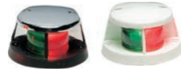
COMBINATION RED-GREEN NAVIGATION LIGHT 12V-5W, 112.5° red - 112.5° green.
