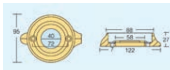
Code 2138 ANODE FOR VOLVO PENTA *851983 Kg 0,485
