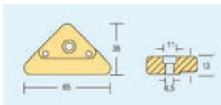
Code 2137 ANODE FOR VOLVO PENTA *872793 Kg 0,120
