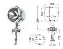
HIGH-BEAM LIGHT ADJUSTABLE FROM INSIDE Made of chromed brass and stainless steel, watertight, adjustable nylon ball joint, frictioning, very small and convenient control handle; supplied with watertight bulbs
