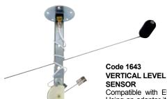
Compatible with EU type 10/189  $\Omega$ . Using an adaptor it can be connected to American type 240/30 $\Omega$  as well. Adjustable length, suitable for tanks with depth 130-660 mm
