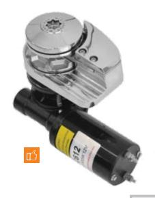
**ELECTRIC WINDLASSES "BARRACUDA"**Powerful and compact windlasses. Parts above deck in high polished stainless steel. Manual free fall with adjustable clutch. Available with handle, solenoid, user manual and mounting guide. Work with chain only or rope/chain combination. The motor can be mounted in all 4 directions.
