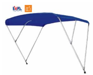
FOLDABLE STAINLESS STEEL CANOPY (with three frames). Provides absolute protection from the sun on small inflatables and crafts. Made of canvas coated by PU, UV resistant and weight 330 gr/m². Its frames are made of st. steel  $\emptyset$  22 mm and are not removable disposing you from the duty of putting them together. Color: Blue.
