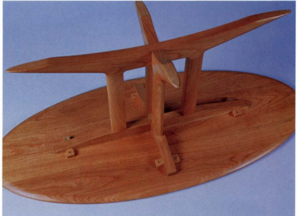
On the underside of the oval table, above, small buttons fit into grooves in the frame to hold the top rigid and flat, yet allow it to move across the grain in response to changes in humidity. A scaled-down blueprint, below, gives students all the information, dimensions and cross-section details they need to build the table.
