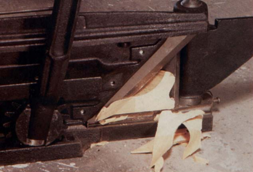
Moldings must be rough-cut to size before the trimmer can start to work. The secret to perfect joints (here with the Grizzly) is to finish up with a series of light slices.
