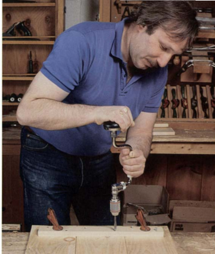
Driving dozens of screws is a breeze with a small-sweep brace, like the 6-in. model shown here. The brace provides more than enough torque for the job, yet provides a sensitive feeling, so screws can be driven to precise depth.
