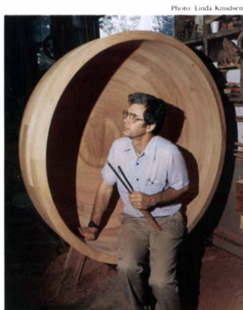
It took Mark Knudsen four and a half days to turn this mahogany bowl, using nothing but a 3/8-in. gouge. The bowl was destined to be cut in half to form two shells atop a 9-ft.-high china cabinet.
