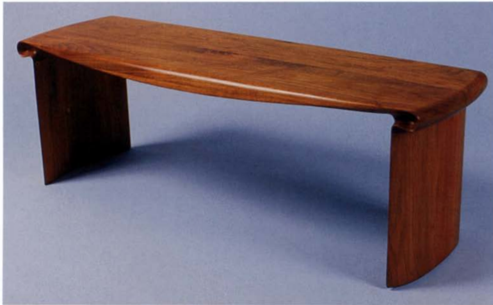
Building the sinuous-line ribbon table requires coopering of the end panels as well as extensive carving of the ribbon-like edges. To build up thickness for the carving, extra wood is glued to the underside of the top around its edges.
