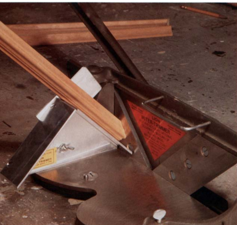
Moldings that tend to tip or tear out when cut normally may be sliced using the Lion's optional top trimmer ($38), which also allows compound miters. Note that the same results can be achieved with a shopmade angled block.
