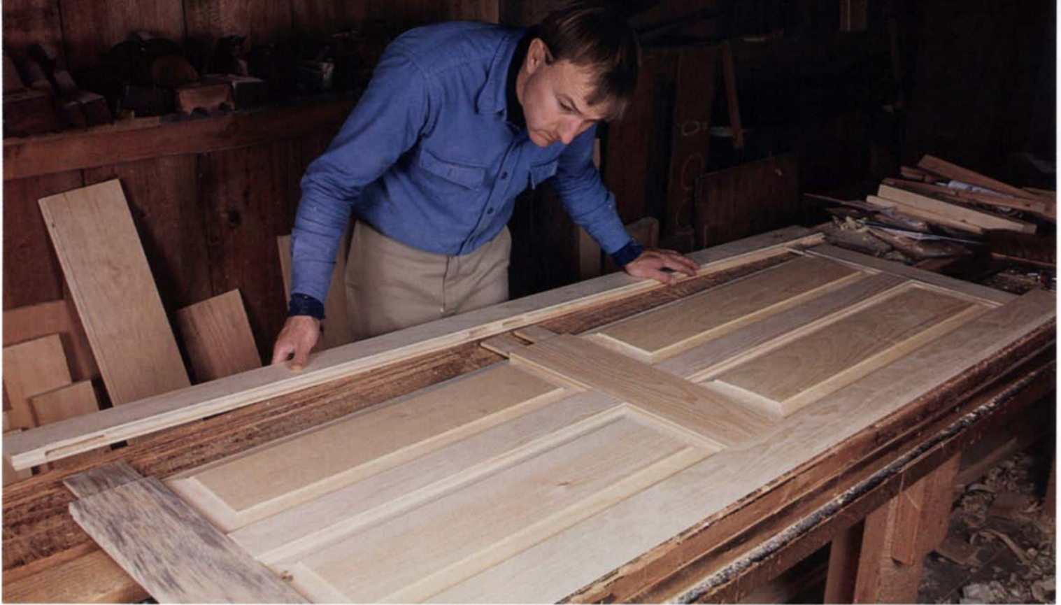
MacGregor's associate, Stu Worthing, assembles the door. Assembly proceeds from the inside out by first inserting the intermediate stiles into the lock rail, followed by the panels and the top and bottom rails. Last in place are the lock and hinge stiles.
