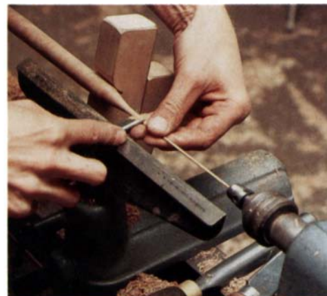
Alan Dorr turns long toothpicks as an exercise in using the skew chisel. This one reached 9 in. before breaking.
