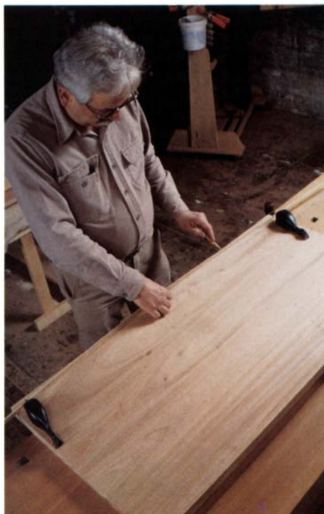
The author uses his spline weights and an oak spline to lay out the curve in the top front of the credenza.
