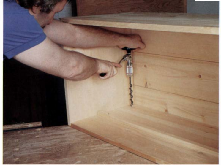
A joist brace, with its ratchet action, can work in spots too tight for even an electric drill. The brace's relatively short height allows it to bore even inside a box, and the long drive handle provides exceptional power to drive the bit.
