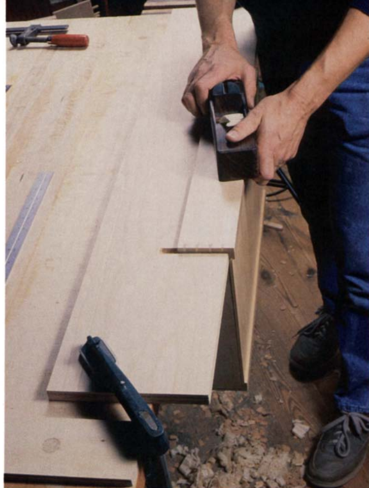
After the glue joints have dried, the drawers are supported on a piece of slotted plywood clamped to the benchtop, then planed to fit. Each drawer is test-fitted and judiciously planed until it slides smoothly. The bottoms are slid in place after the drawers are fitted.
