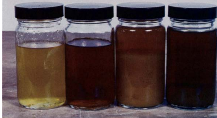
Shellac can be refined to various grades. From the left: bleached, dewaxed; dewaxed blonde; Kusmi Superior; Siam seedlac. Note that shellacs containing wax will appear cloudy and may settle into strata with hard resin on top.
