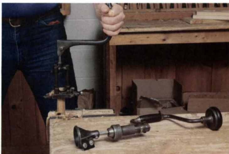
After chamfering the end of a chair rung with a spoke pointer, fitted in the brace in the foreground, the author uses an adjustable hollow auger to form a tenon on the rung. A plane-like blade on the bottom of the auger cuts the tenon by paring a shoulder around the tenon.
