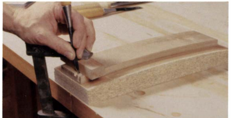
The author leans the chisel against an angled guide block while chopping waste from the pins in the drawer's front. The front is clamped on a piece of glued-up particleboard bandsawn to match the curve of the front. Sandpaper glued to the block stops the front from slipping.
