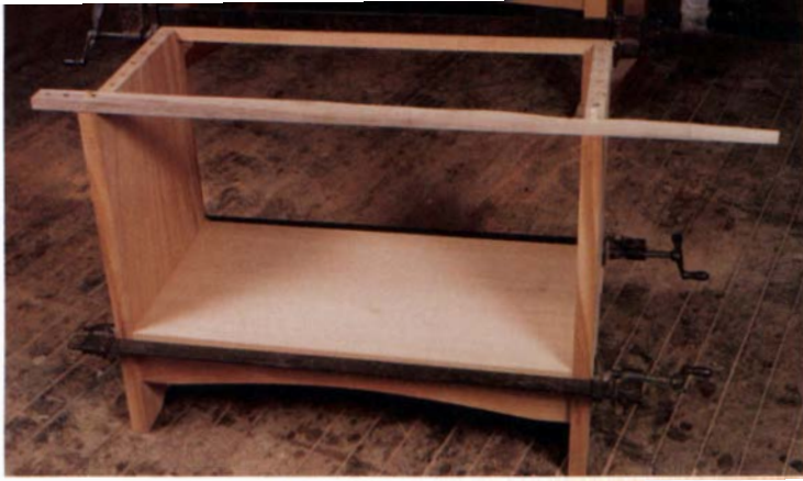
A temporary glue-up stick attaches over the dowels at the top to keep the sides from toeing in or out as glue dries.
