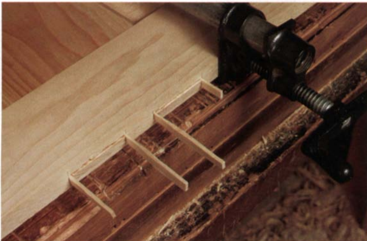
Above, wedges and pins lock the tenons securely without glue. The wedges are driven in above and below the tenons until they seat firmly. Below, pins made from rounded square stock are driven into 1/4-in. through-bored holes.
