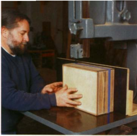
Saw the top off the box on a band-saw. Tape the entire saw line, and use a 1/2-in., 3-tpi blade to avoid breakout.
