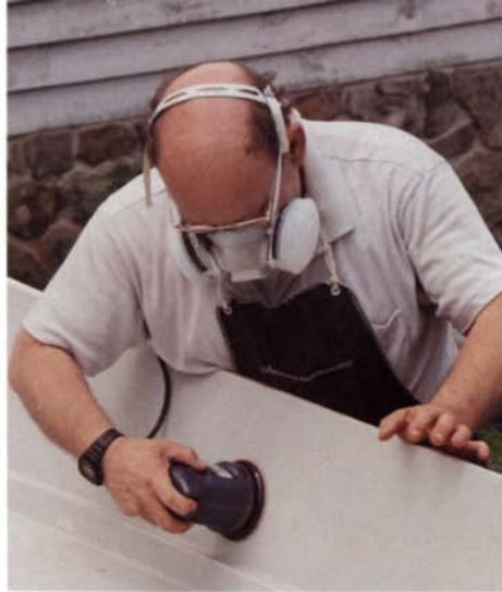
Half-face mask —These respirators are usually made of soft rubber or silicone and have replaceable filter cartridges.
