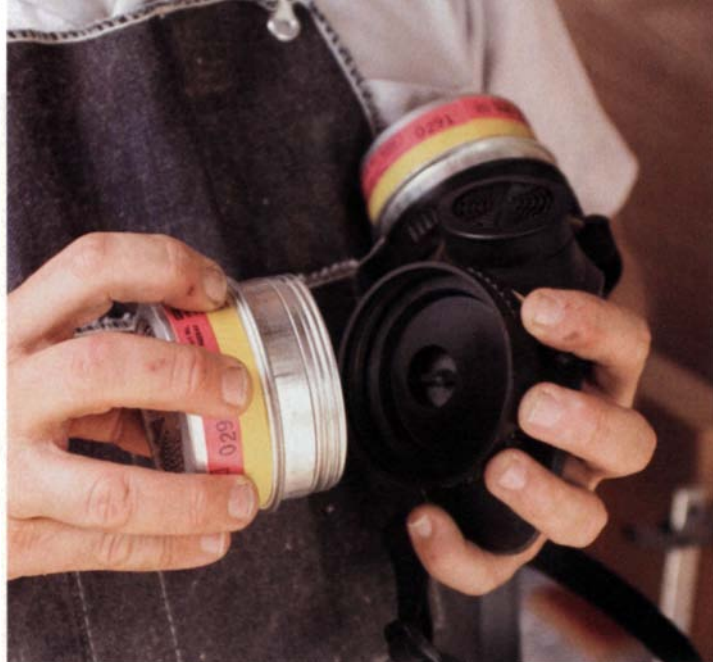
Use the proper cartridge for the chemical hazard. For spraying lacquer, organic vapor cartridges, which contain carbon filters, will trap hazardous fumes.
