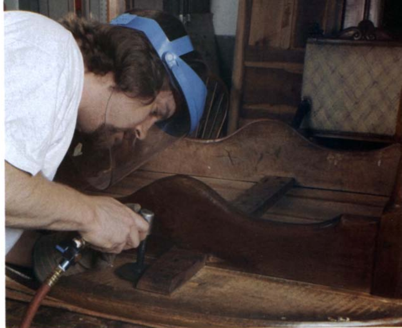
Spoil the nails and spare the table. After carefully prying up the batten on the underside of a table, the author uses a large cutting wheel to cut through rusted nails.
