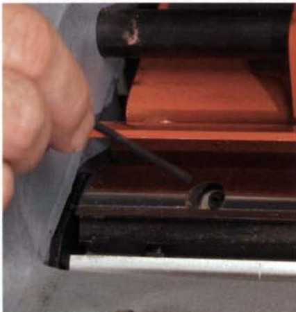
Cutterhead with jackscrews —Knives rest on adjustable jack screws; gib and gib screws keep knives in place.
