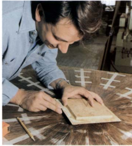
Trammel center must be positioned precisely. The author lines up the corners of the laminate on seams of the sunburst pattern, automatically centering the fixture.
