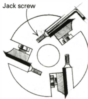
Cutterhead with jackscrews —Knives rest on adjustable jack screws; gib and gib screws keep knives in place.
