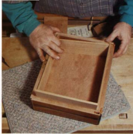
Gently press-fit lining around interior. When you season the humidor, the lining will swell and lock itself in place.
