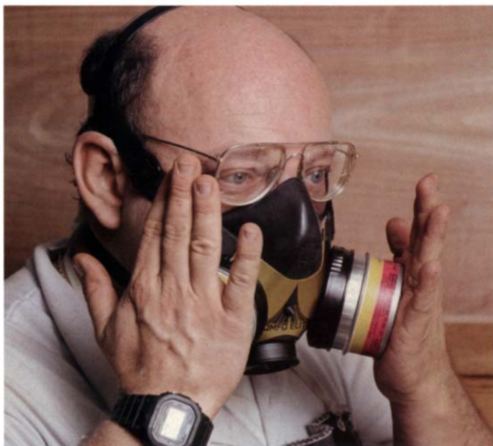
Testing the fit of a cartridge-style respirator —Cover the cartridges with your hands and inhale. The vacuum pressure created should collapse the mask against your face.
