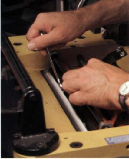
Typical cutterhead —Knives rest on springs and are held in place by gibs and gib screws.
