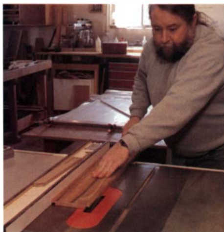
Rabbet the four sides at once, while they're still one piece. A dado blade will make the cut in one pass.
