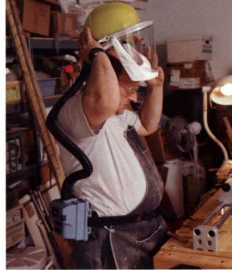
Full-face protection —Powered air-purifying respirators deliver a constant supply of filtered air.
