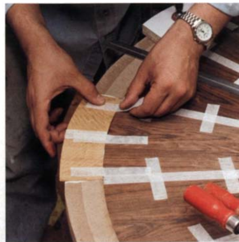
Tape crossbanding in place. After spreading glue in the rabbet, stick veneer tape to the crossbanding, and pull it in toward the center.
