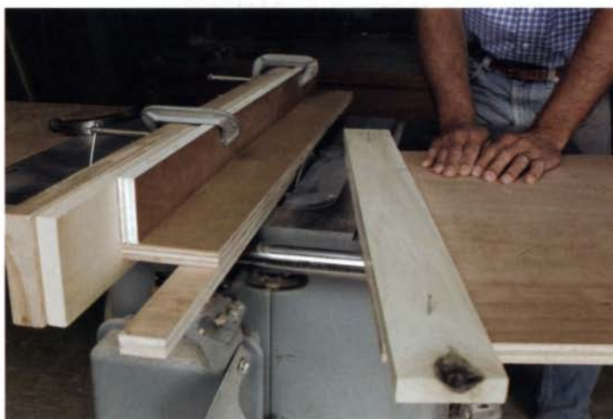
3. Leave plenty of space between blade and saw fence to prevent the offcut from binding.
