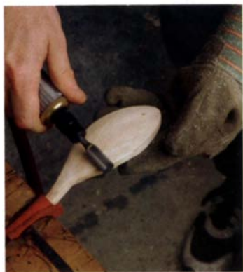
A carbide burr roughs out a spoon blank in no time. Burrs grind wood more than they cut it. This makes them easy to handle for freehand shaping. Wear gloves: If you ever touch a spinning bit, you'll know why.
