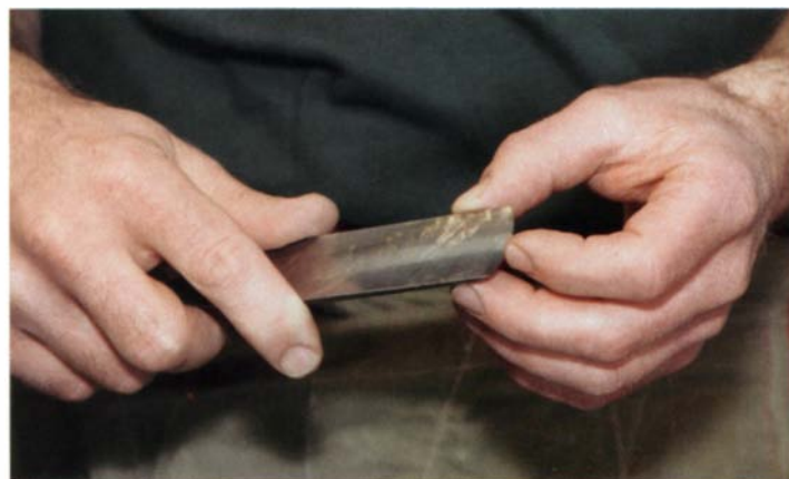
The author uses a fingertip to judge blade sharpness. A finger passed lightly over a razor-sharp tool will drag smoothly. Catches indicate rough spots.
