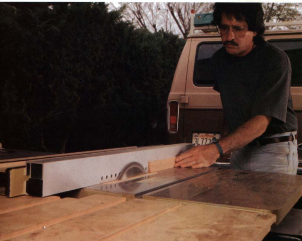
Ripping made safer—The Vac-U-Fence attaches to a stock rip fence. A shop vacuum provides suction to hold stock steady when ripping.
