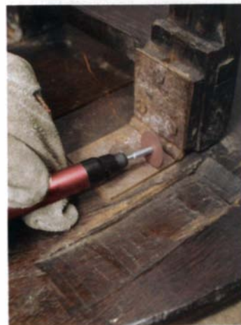
Cut a new slot in an old screw. Without marring the hinge, a microgrinder fitted with a thin grinding wheel cuts a short, deep slot.
