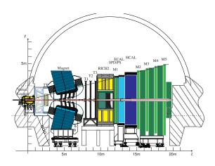
Figure 1: Vertical cross section through the LHCb detector. The LHC proton beams collide inside the Vertex Locator on the left.
