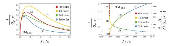
Figure 3: Plots of the 0th, 1st, 2nd and 3rd order approximations of  $1/Q_{\gamma'}$  (solid line) and its derivative (dashed line) against frequency / threshold frequency for the TM<sub>010</sub> mode in a cylindrical cavity of unity aspect ratio (L = 2R) with tuning performed by changing the size of the cavity whilst maintaining the aspect ratio.
