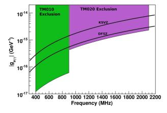
Figure 2: Target exclusion region for  $TM_{010}$  and  $TM_{020}$  modes of ADMX Phase 2 with dilution refrigerator installed after one year of running.
