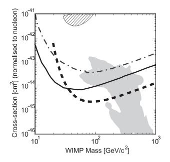
Figure 1: Measured and expected sensitivities of WIMPs-nucleon cross section as a function of WIMP mass. Hatched region is  $3\sigma$  arrowed region by DAMA/LIBRA with no ion channeling[3]. Shaded region is a result of a theoretical calculation in [4]. Upper region of a solid thin line and a line-dashed lines are excluded by XENON100[5] and CDMS[6], respectively. XMASS expected sensitivity is plotted in thick dash line.
