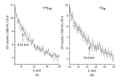
Figure 2: The Si(Li) detector energy spectra of  $^{169}$ Tm (a) and  $^{57}$ Fe (b) targets, measured in the anticoincidence with the veto signal. Solid line shows the fitting results for corresponding regions.
