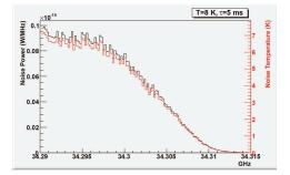
Figure 1: Noise power (top line) and noise temperature (bottom line) of the signal cavity.
