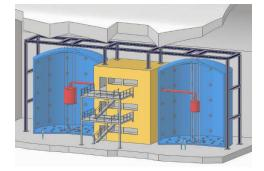
Figure 3: Illustration of a possible layout of the DARWIN facility: A 10 ton LXe detector (5 ton fiducial mass) and a 20 ton LAr detetector (10 ton fiducial mass). In the final realization, the two detectors do not necessarily need to be placed directly next to each other.
