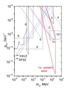
Figure 3: The limits on  $g_{A\gamma}$  obtained by 1- present work (a -  $A \rightarrow 2\gamma$ , b - PC, areas of excluded values are located inside contour), 2 - CTF [1], 3- reactor experiments, 4- beam dump experiments, 5- resonant absorption [13], 6- solar axions conversion in crystals, 7- CAST, 8- telescopes, 9- HB Stars, 10-expectation region from heavy axion models.
