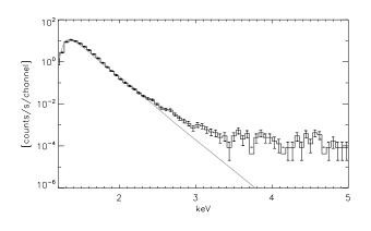
Figure 1: The SphinX solar X-ray spectrum measured for a very low activity period. The best isothermal model fit folded with DRM is shown in dashed line
