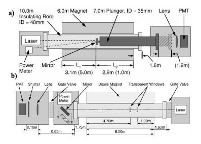
Figure 1: (a) Schematic diagram of the (a) GammeV experimental apparatus and (b) GammeV-CHASE experimental apparatus. The laser, spare Tevatron magnet, phototubes, and data acquition electronics were used by both experiments.
