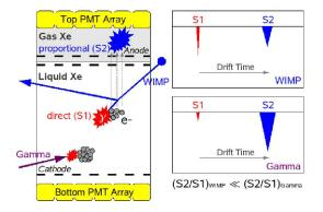
Figure 1: Principle of a two-phase liquidnoble gas TPC: Interactions generate prompt scintillation light (S1) and ionize the liquid target. The ionization electrons (charge signal, S2) are drifted upwards and detected in the gas volume. The event vertex is reconstructed from the S2 pattern and the electron drift time. The S2/S1 ratio is used for signal/background discrimination. In LAr, the S1 pulse-shape provides another powerful discrimination channel.
