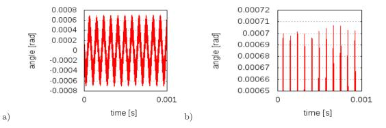
Figure 2: a) The angle between the spin and momentum vectors for  $dp/p = 2 \times 10^{-4}$  and 28 m of total straight section length. b) Zoom-in the top region of (a) shows that the angle fluctuates but remains constant to about  $0.25 \times 10^{-5}$  radians over 1ms.
