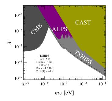
Figure 2: Current exclusion regions for hidden photons with kinetic mixing angle  $\chi$  and mass  $m_{\gamma'}$ , in particular from the light-shining-through-a-wall experiment ALPS and from the helioscope experiment CAST, together with the projected sensitivity of TSHIPS (gray region).
