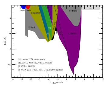
Figure 3: Preliminary exclusion limit for hidden photons as a result of the non observation of a signal in the measurement-run from the 11/2011 at CERN (labeled as [2]), compared to the result of other experiments. The collection of experimental data has been taken from [3], where it is also explained in detail.
