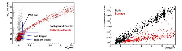
Figure 3: (a) Left: Scattered plots of the  $SA_6^P$  (shaping time 6  $\mu$ s with partial integration) versus  $SA_{12}^T$  (shaping time 12  $\mu$ s with partial integration) signals, for both calibration and physics events. The PSD selection is shown. (b) Right: Rise time plots, as characterized by the amplitude of timing amplifier (TA) signals, showing different behaviour between surface (faster) and bulk (slower) events.
