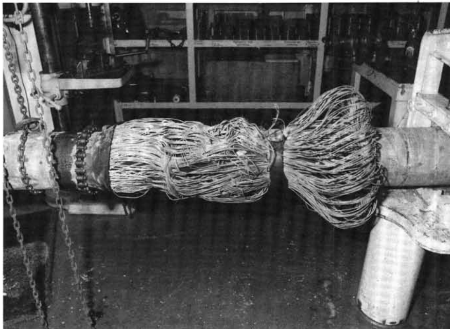
Figure 59. Photograph of TAM drill-in packer after deployment in Hole 671C. Note that most of the rubber that originally covered the braided metal cable was stripped away during drilling.
