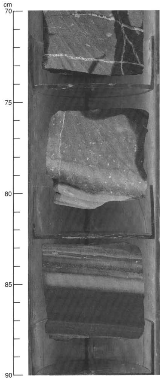
Figure 42. Piece in center includes contact between chilled marginal facies of Unit 7 and baked sediments at the base of the unit. Section 127-797C-19R-4 (Piece 8).
