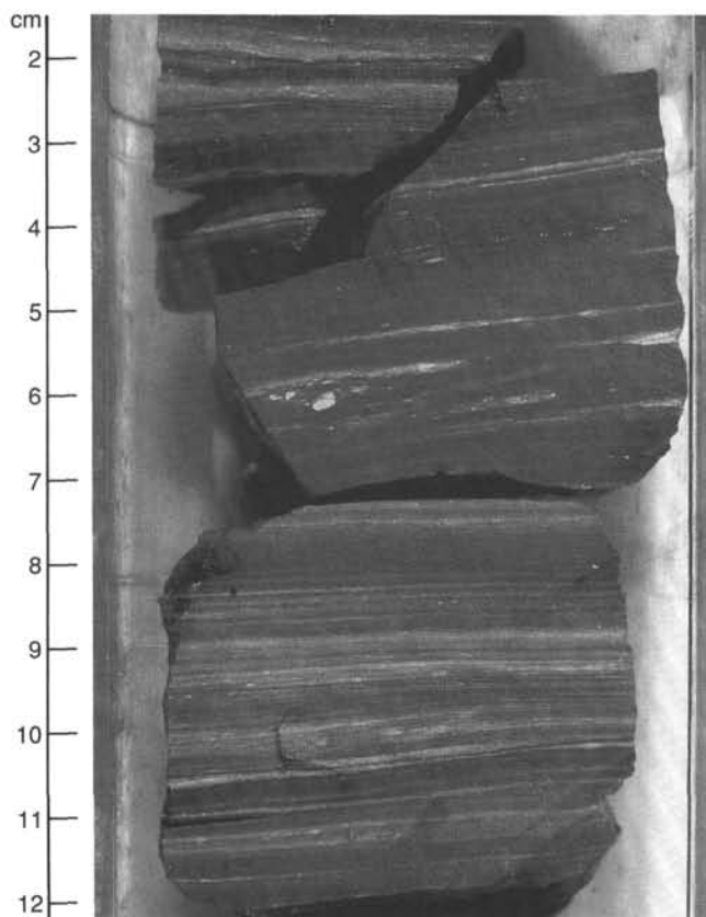
Figure 43. Section 128-799B-45R-2 at 2–12 cm illustrates well-developed laminations and elongated nodules of diagenetic carbonate in dark porcellanite; scattered sand-sized glauconite grains are evident in the upper several centimeters of the photograph.
