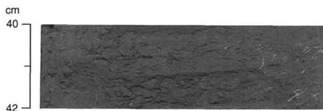
Figure 27. Interval exhibiting a very thin zone of scaly fabric, interval 156-948C-16X-6, 40-42 cm.
