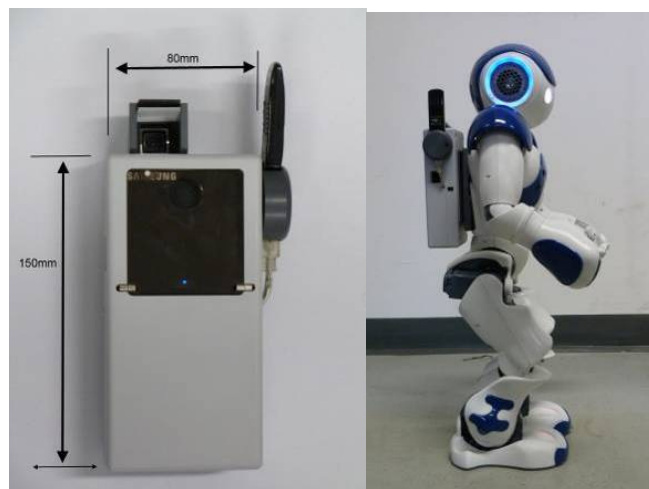
Figure 1. Prototype of LED projector unit (left) mounted on the humanoid NAO robot (right)
