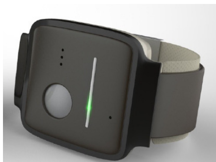
Figure 2. Okkolo is a bracelet controlling user's health condition. It will inform a caregiver automatically and immediately on user's health change: pulse rate, temperature, falls
