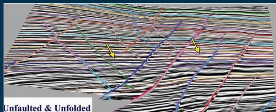
Figure 1 – Data example 1; vertical and horizontal scales are not defined. Yellow arrows indicate thinning oil-filled sands.
