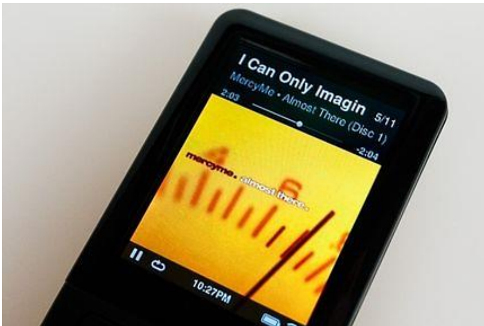
The Now Playing view ; album art, album name, track number, song name, song progress, time, battery life, Wi-Fi connection, play/pause status, and repeat on/off...a lot of information at a glance !
