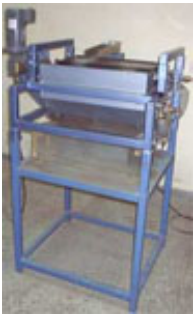
High intensity permanent magnetic rolls
