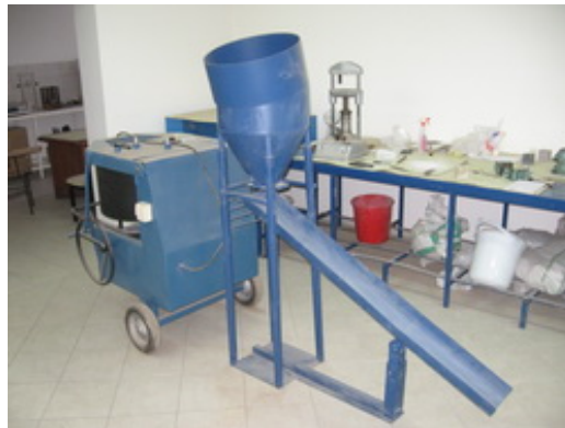
Concrete mixer and segregation apparatus
