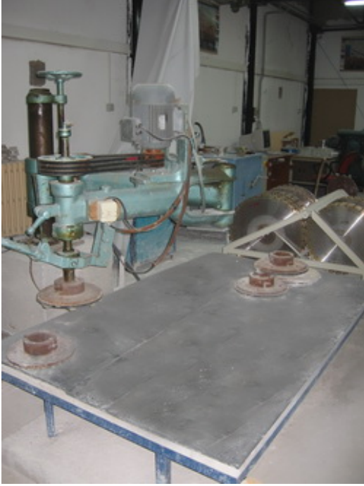
Surface polishing equipment
