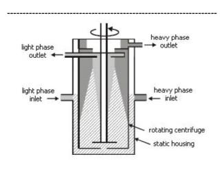
Fig. 1. Cross-sectional view of the CCCS. Hatched: dispersion, light grey: light phase, darker grey: heavy phase
