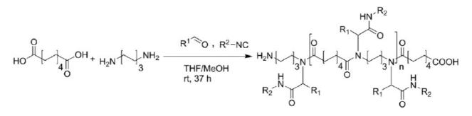
Figure: One of the possible combinations for the polyamide synthesis *via* the Ugi-4CR employing a renewable dicarboxylic acid.
