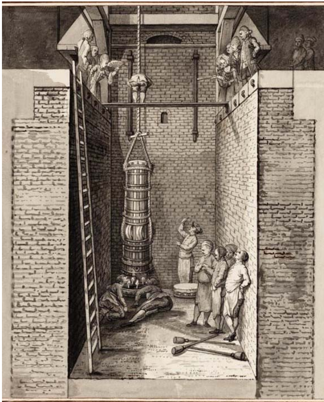
Fig. 8.: Making of a gun-founding mould. (Carel de Beer: The Art of Gunfounding)
