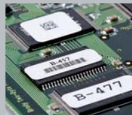
Circuit Board Labeling
