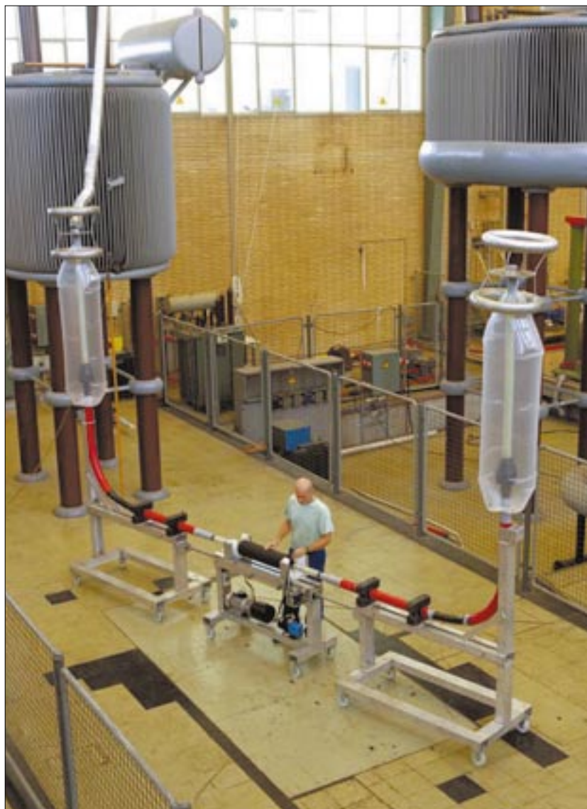
An image of the Click-fit joint in the Dutch factory.
