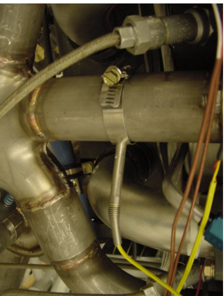
EGT Probe Location
