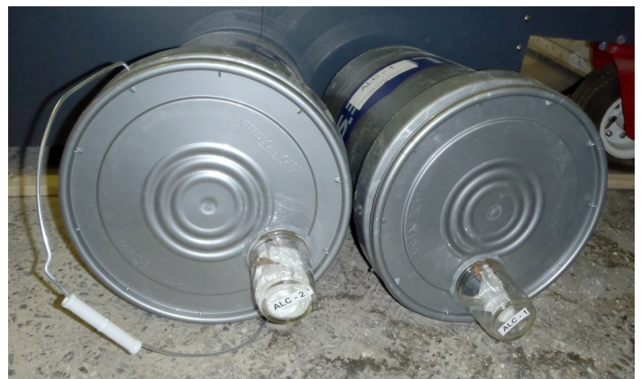
Figure 5: A rearing chamber made from five-gallon plastic buckets, designed to capture wood borers emerging from firewood. Photo by Mia Kirk, AK DNR.
