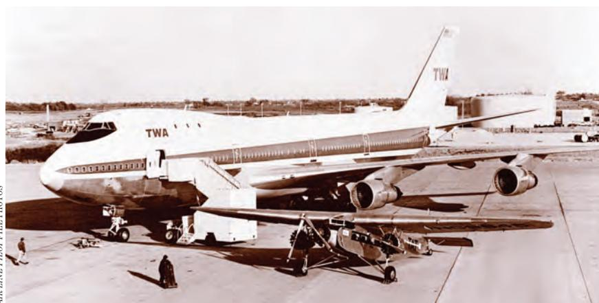
***A Ford Trimotor with TAT markings sits aside a TWA jumbo B-747 in a graphic display of equipment growth at T&WA/TWA. The Trimotor took 36 hours to make the coast-to-coast flight; the B-747 takes 6.***
