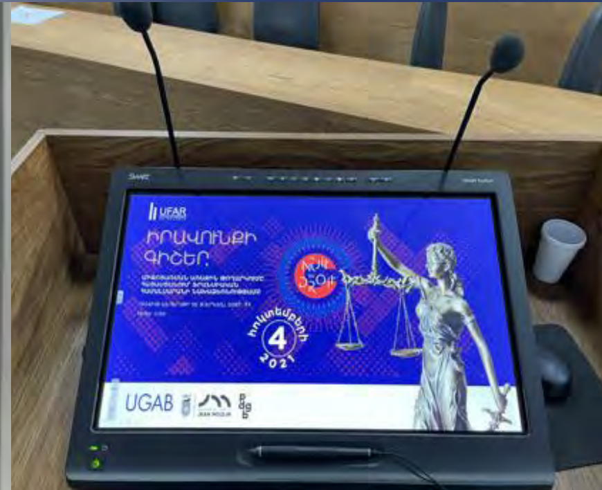
SMART Podium 524 Interactive Pen Display – 1 pcs: ( 24" (61 cm) diagonal, native Full HD (1,920 x 1,080) res-n, Battery-free tethered pen with a comfort grip; Adjustable stand)
