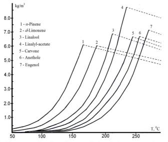
Fig.1. Temperature dependence of the vapor density of basic components of essential oils
