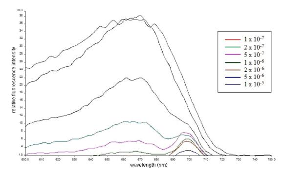
**Figure 3.** The fluorescence spectra of  $10^{-4}$  M ascorbic acid and MB (emission spectra  $\lambda_{em} = 694$  nm) depending on MB concentration.
