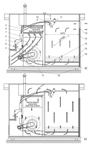
Figure 1 Experimental dryer, a) open mode, b) circulating mode
