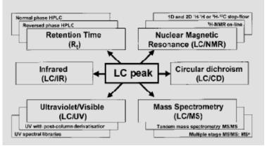
**Figure 1.** Type of information that can be obtained from a given LC peak using the different LC coupled (hyphenated) techniques available. [1].
