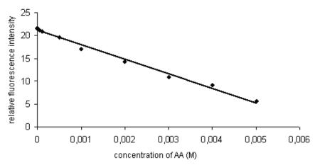
Figure 5. Calibration curve – relative fluorescence intensity was measured after 5 minutes for different concentrations of AA.
