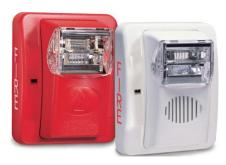
Audio-visual alarm devices are used as general fire alarm annunciation devices as part of building fire alarm systems, and they are also typically installed inside the protected space that is being protected by a Stat-X fire suppression system. AHJs can also require these devices to be provided outside each point of egress from a space that is protected by a Stat-X fire suppression system.
