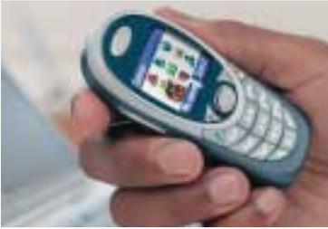
The next generation of mobile phones will offer far greater functionality and bandwidth. Here no manufacturer can avoid higher scales of integration, because next-generation handsets put together from discrete components with conventional circuit technology would be several times larger and heavier than today's mobile phones.
