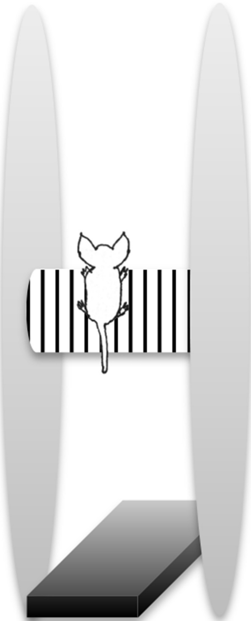
Figure 1. Schematic representation of the rotarod (Mouse RotaRod NG, model 47650, by UgoBasile). The animal walks on a rotating cylinder with progressive acceleration. The two circular panels prevent the animal jumping out of the way. A tub is placed with a padded cushion under the rod to secure the animal in case of a fall (the height from the tub to the base of the rod is 21 cm) so that the animal would not be hurt.
