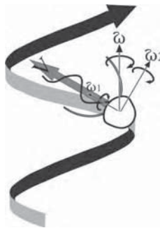
FIGURE 13.12 Swimming in a helix, in this case for the flagellate Pteridomonas . The swimming path of the organism and hence the helix is defined by the velocity vector ( V ) and the rotational vector ( \omega ). is a sum of a component ( \omega_1 ) parallel to the velocity vector and a component ( \omega_2 ) perpendicular to the velocity vector. The axis of the helix will be parallel to \omega .
