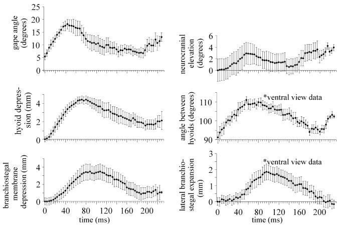
**Fig. 6** Mean kinematic profiles, with standard error bars, of selected kinematic variables during prey capture in one individual *Clarias gariepinus* (cranial length=46.10 mm, total length=182.20 mm). Ten
