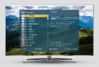
Electronical program guide provide users of television with continuously updated menus displaying broadcast programming or scheduling information for current and upcoming programming. User can choose between vertical horizontal and multi-channel EPG.
