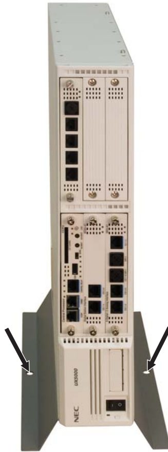
Figure 1-73: FLOOR MOUNTING 1 CHASSIS-A
