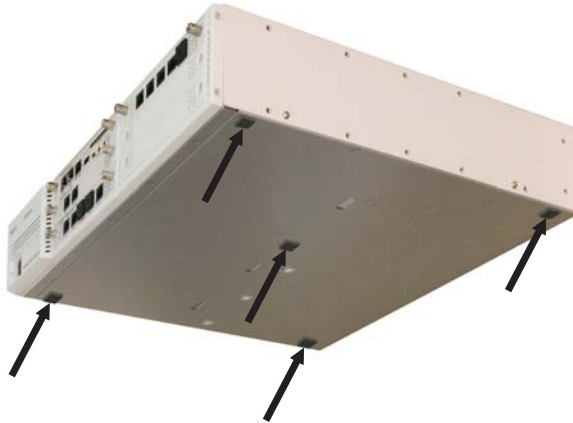
Figure 1-74: ADD RUBBER FEET FOR MULTI-CHASSIS INSTALLATIONS
