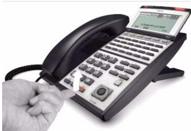
Figure 4-31: REMOVING THE FACEPLATE
