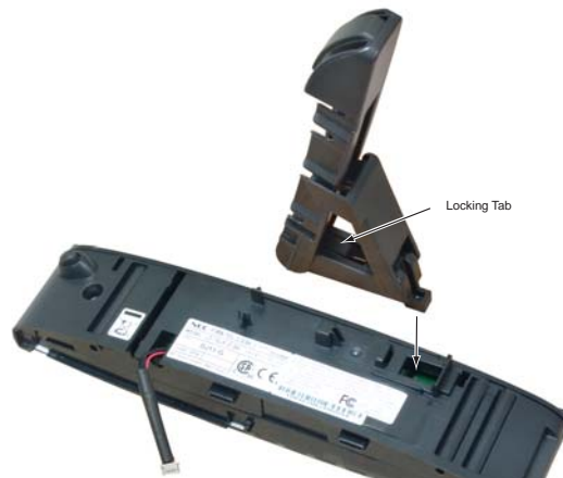
Figure 4-36: ATTACHING THE TERMINAL LEG(S)
