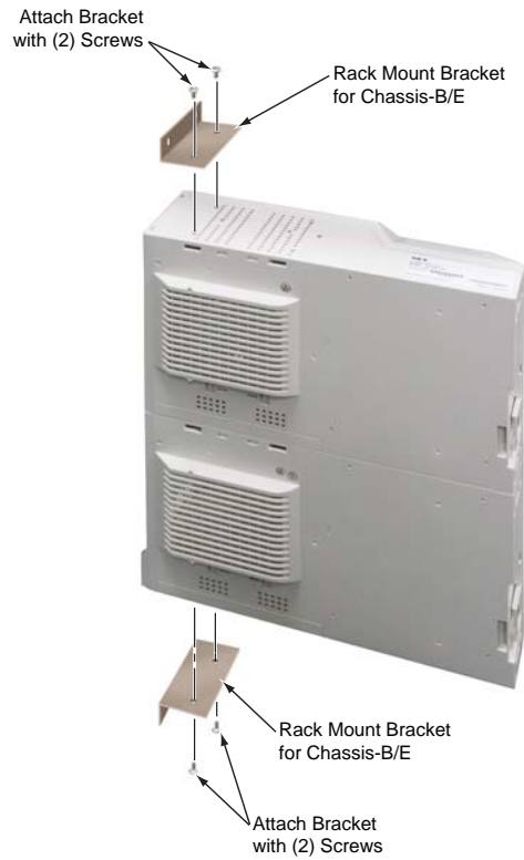
Figure 1-88: ATTACH RACK MOUNT BRACKETS TO CHASSIS-B/E
