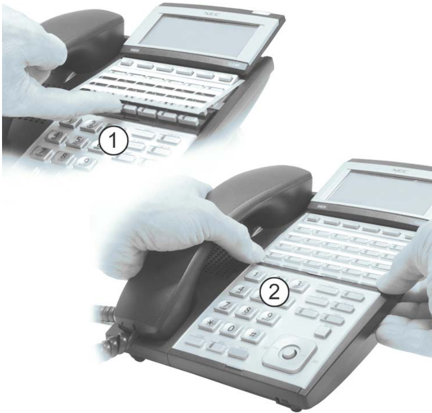
Figure 4-32: REPLACING THE FACEPLATE
