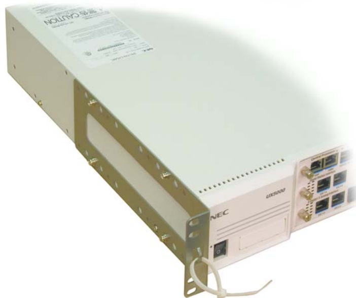
Figure 1-89: ATTACH RACK MOUNT BRACKETS TO CHASSIS-A
