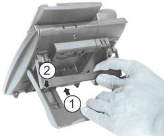
Figure 4-34: INCREASING THE TERMINAL HEIGHT
