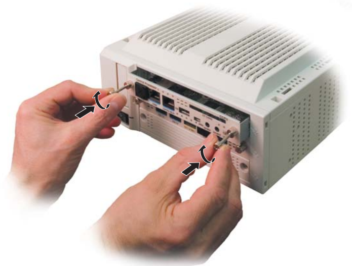
Figure 2-7: TIGHTEN THUMB SCREWS
