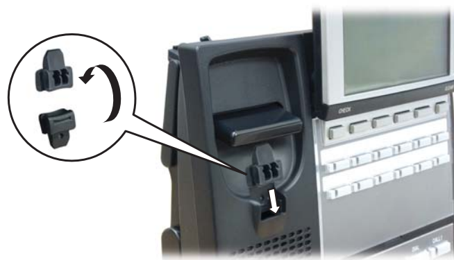
Figure 4-39: INSTALLING THE HOOKSWITCH HANGER
