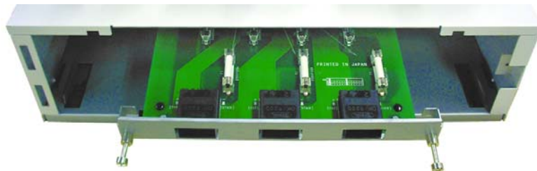
Figure 1-42: REMOVE FUSE BOARD
