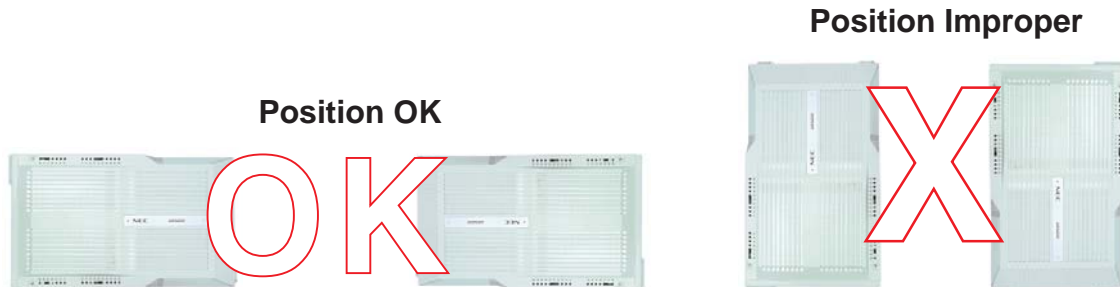
Figure 1-44: WALL MOUNTING POSITION FOR CHASSIS-B/E
