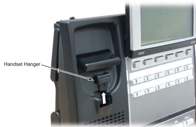
Figure 4-38: REMOVING THE HOOKSWITCH HANGER
