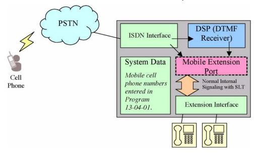
The number of Mobile Extensions per UX5000 is based on the number of extension ports in the UX5000. For smaller systems, it is important to remember that the number of Mobile Extension ports = 25% of physical ports (8 ports allows for 2 Mobile Extension entries).
