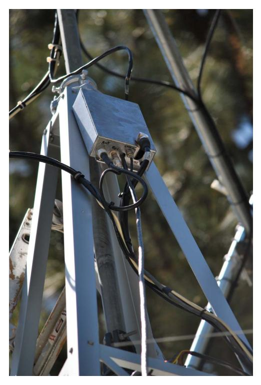
This Figure shows the mast-mounted box containing the pre-amp and two relays. The large relay inside the box connects the antenna array to the Heliax and the smaller relay connects the array to the pre-amp input. During transmit the small relay switches a 50  $\Omega$  termination to the pre-amp input. The pre-amp is connected to the transceiver with a RG8X cable run.
