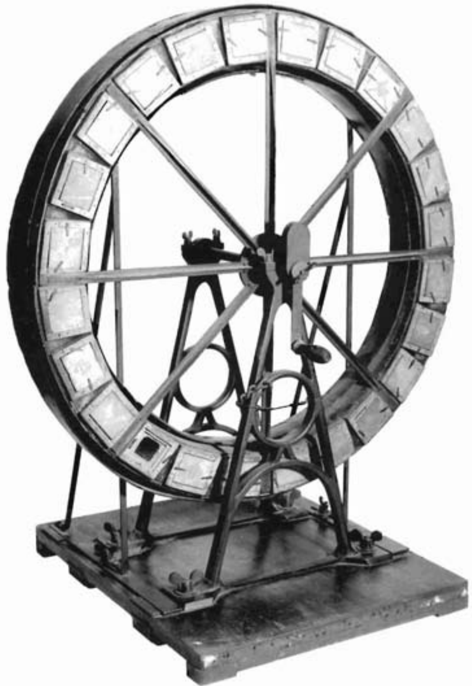
Figure 3 Kohlrausch's first chronophotographic apparatus, 1890, seen from the back, with 24 negative mounts attached to a movable wheel operated by a hand crank. (Deutsches Museum)
