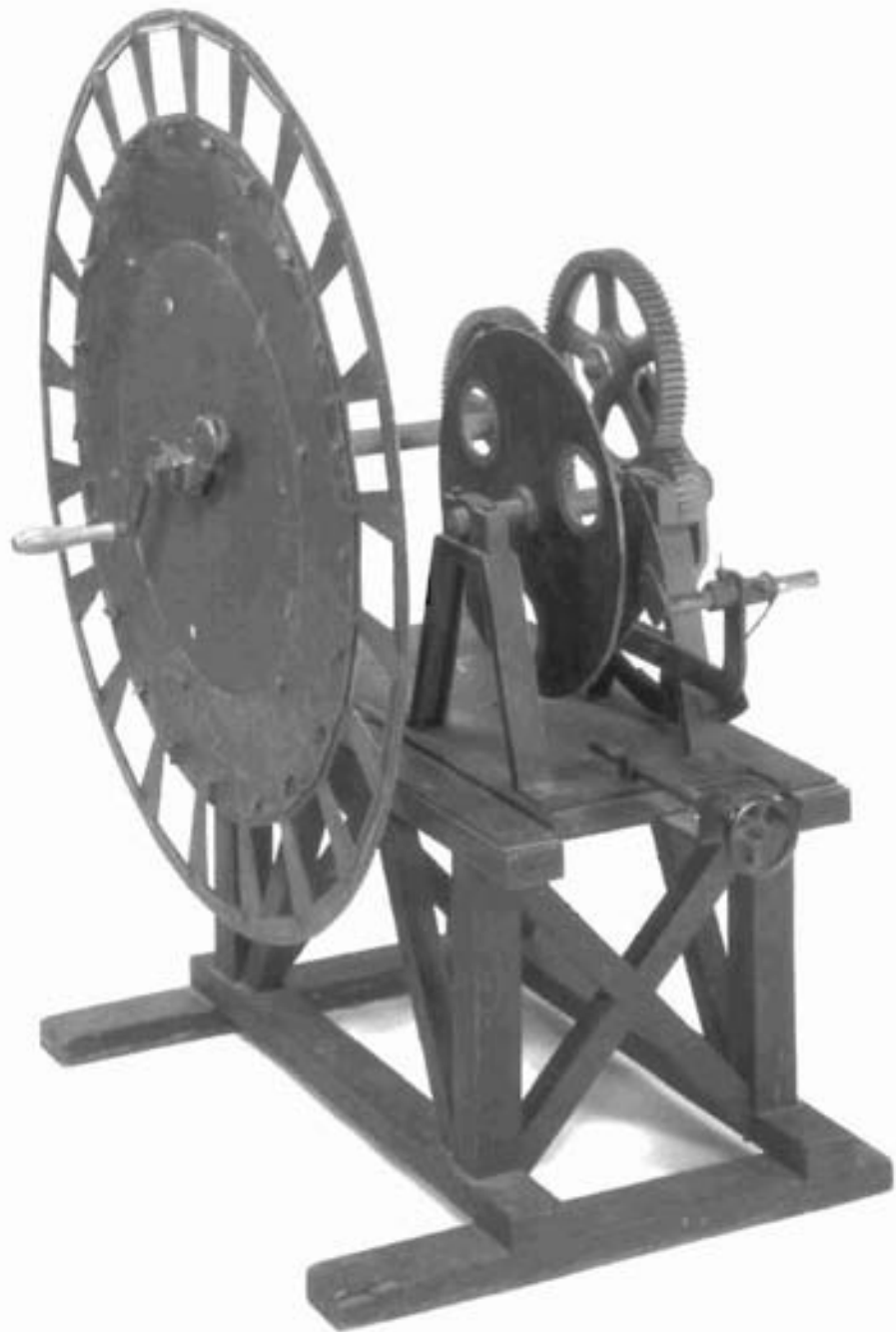
Figure 8 Kohlrausch's first projecting apparatus, 1892/93, three-quarter view from the back, showing the hand crank, the disc for 21 lantern slides and the disc for the lenses behind it. (Deutsches Museum)
