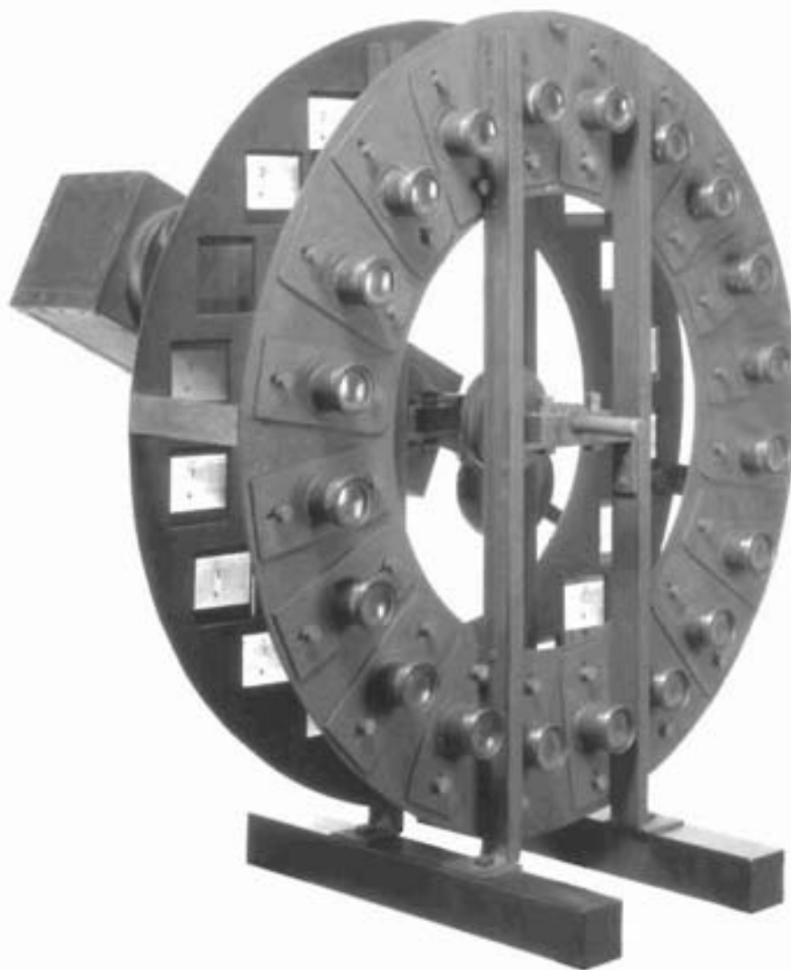
Figure 9 Kohlrausch's second projecting apparatus, 1895, front view, showing 20 lantern slides on a fixed ring and a movable 'arm' behind it for introducing light. (Deutsches Museum)
