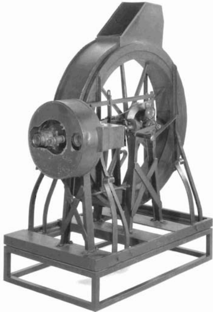
Figure 6 Kohlrausch's second chronophotographic apparatus, 1892, three-quarter view from the front, showing encased wheel with lenses perpendicular to the large wheel with 25 negative mounts operated by a hand crank. (Deutsches Museum)
