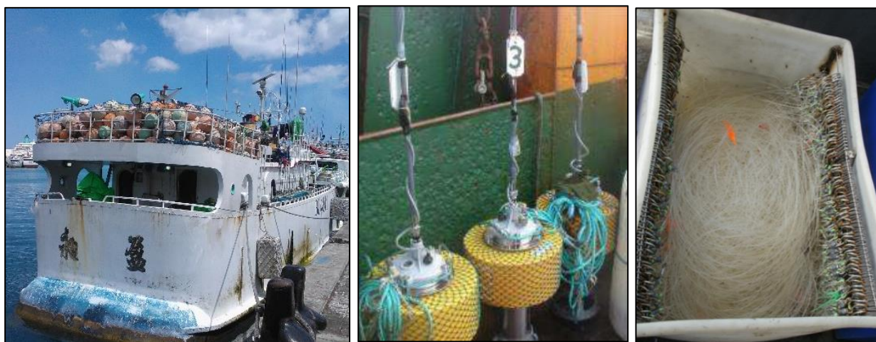
Figure 29: Photographs showing marker buoys (left), radio buoys (centre) and monofilament branch lines (right) (Source: CapMarine, 2015).
