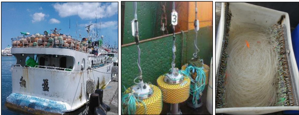
Figure 4-22: Photographs showing marker buoys (left), radio buoys (centre) and monofilament branch lines (right) (Source: CapMarine, 2015).
