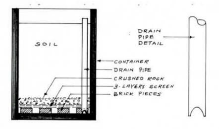
the pot bottom, evenly spaced. The surface must be as level as possible. Next, cut two pieces of 1/4 inch or 1/2 inch galvanized hardware cloth to fit the inside of the container. This is obtainable at any hardware or building supply store. On top ot this double layer, place a piece of plastic household screen, cut to fit. never use copper or bronze screen for this layer.
