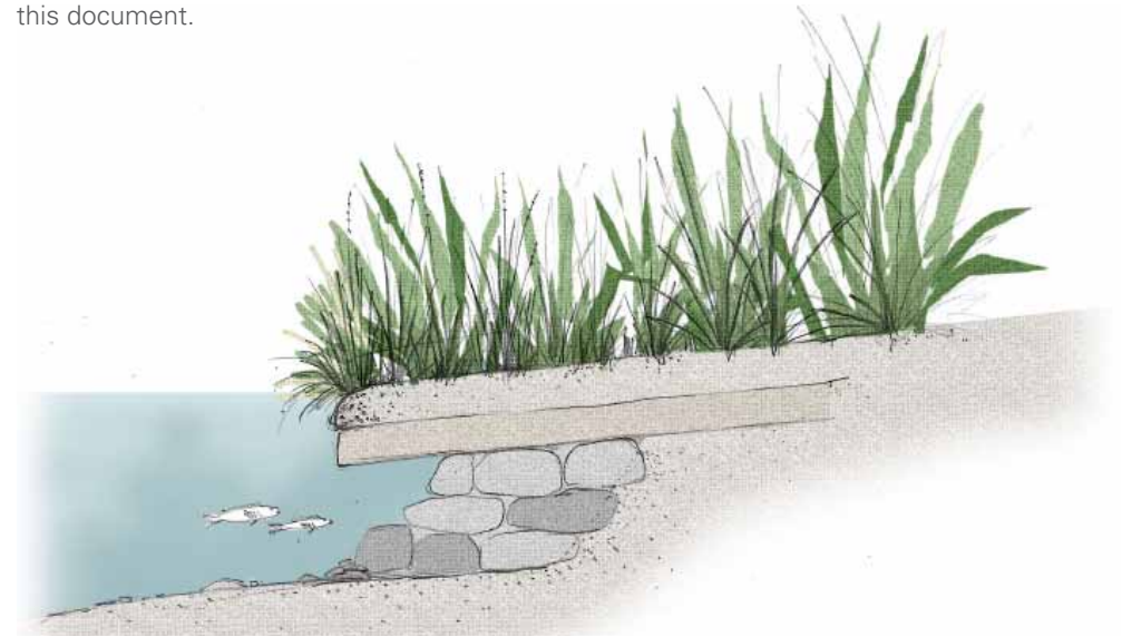
Figure 53: Potential to construct temporary fish refugia until plants can establish and maintain overhanging structures
