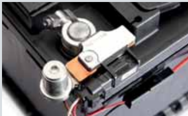
Mounting on standard battery pole (battery pole adapter not included in delivery)
