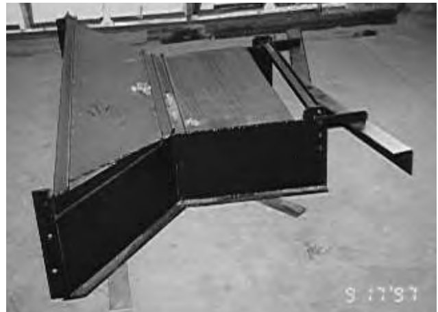
Fig. 8.2. Bed builder, which attaches to tractor with three-point hitch, for forming mounds in deep soil or rocky soil. Not commercially available. This one was constructed by a welder.
