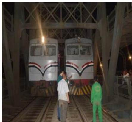
Figure 16: Locomotive test position at field test of Imbaba Railway Bridge.
