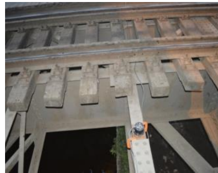
Figure 12: piezoelectric accelerometers. Figure 13: Accelerometer attached on the cross girder of the bridge.
