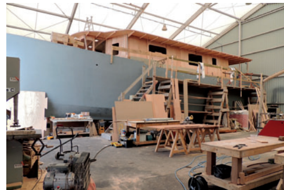
The choice of plywood laminated with glass-epoxy was logical for the construction of Etoile 65...
