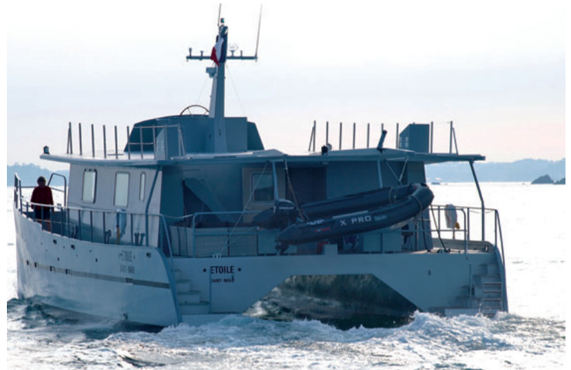
With 1.4m under the bridgedeck, the cat never slams, even in (very) rough conditions, such as those we encountered during our test.
